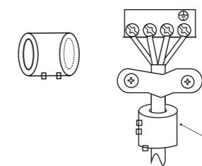
Pass the belt through the hole of the Magnetic ring to fix it on the cable
