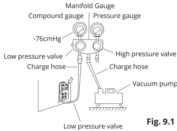
1. Connect the manifold gauge's charge hose to the service port on the outdoor unit's low pressure valve.
