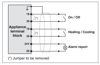
The control cable should go into the appliance through a grommet (not supplied - drilling to be made).
