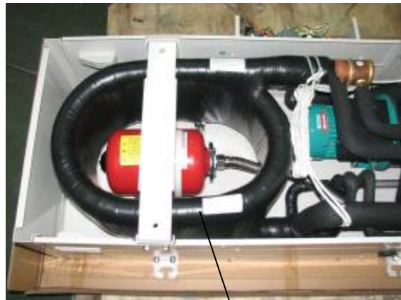
Tube in tube heat-exchanger
