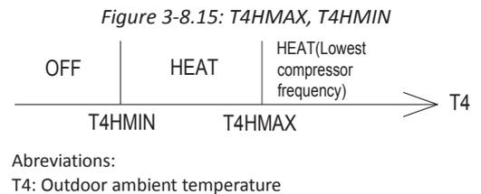
**T4HMIN** sets the ambient temperature below which the heat pump will not operate in heating mode. The lowest value that **T4HMIN** can take is -25°C, which is the heating mode lower ambient temperature operating limit of the heat pump. Refer to Figure 3-8.16.
