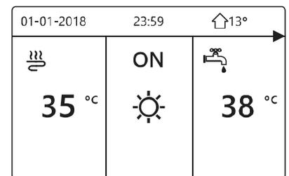
**ROOM TEMP.** sets whether space heating/cooling modes are controlled according to the room temperature detected by the temperature sensor in the Matrix Split user interface. If **YES** is selected, the user is able to set the room temperature set temperature on the user interface’s main screen, no matter what is the setting of **WATER FLOW TEMP.**
