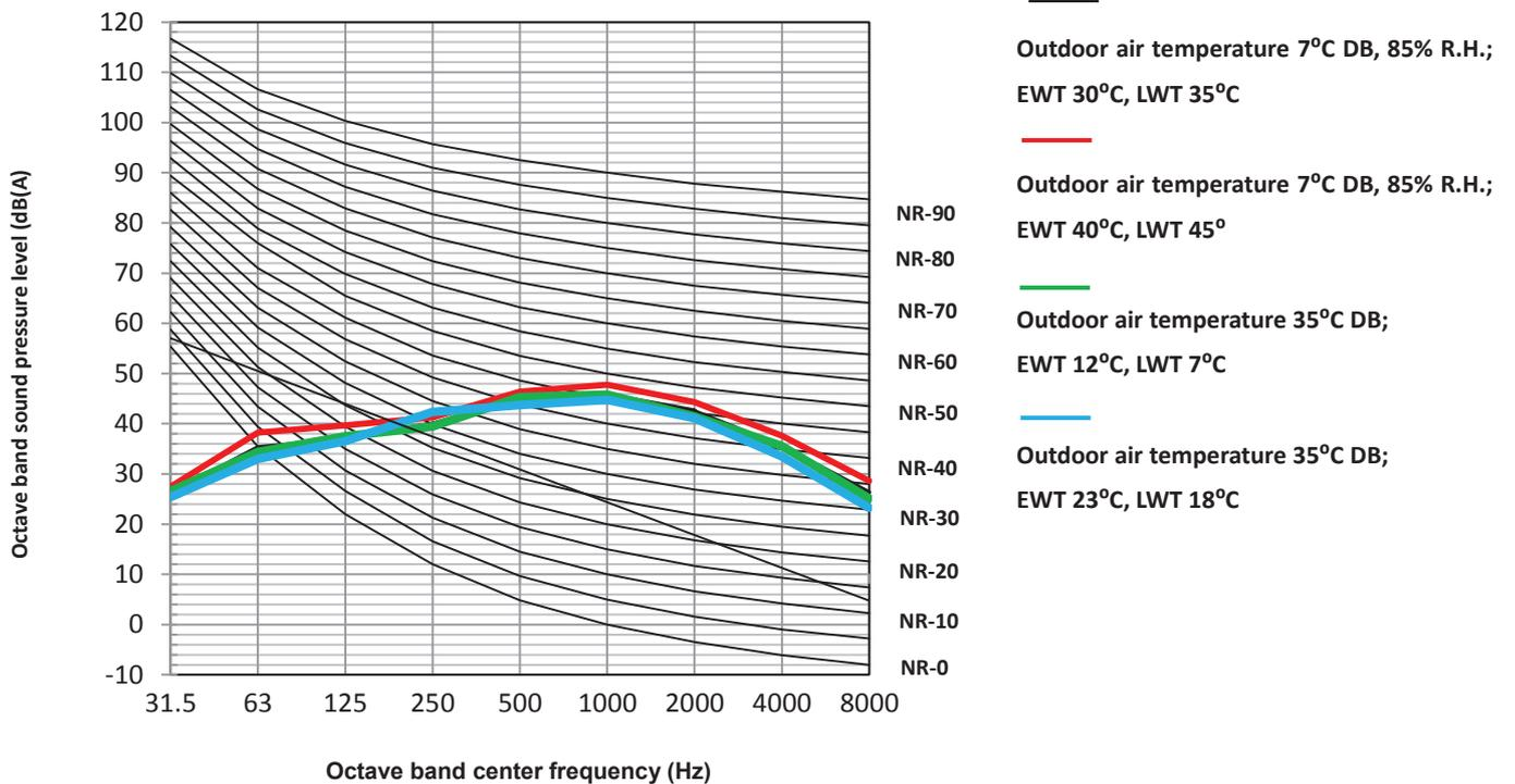
Figure 2-8.5: ATS12S octave band levels
