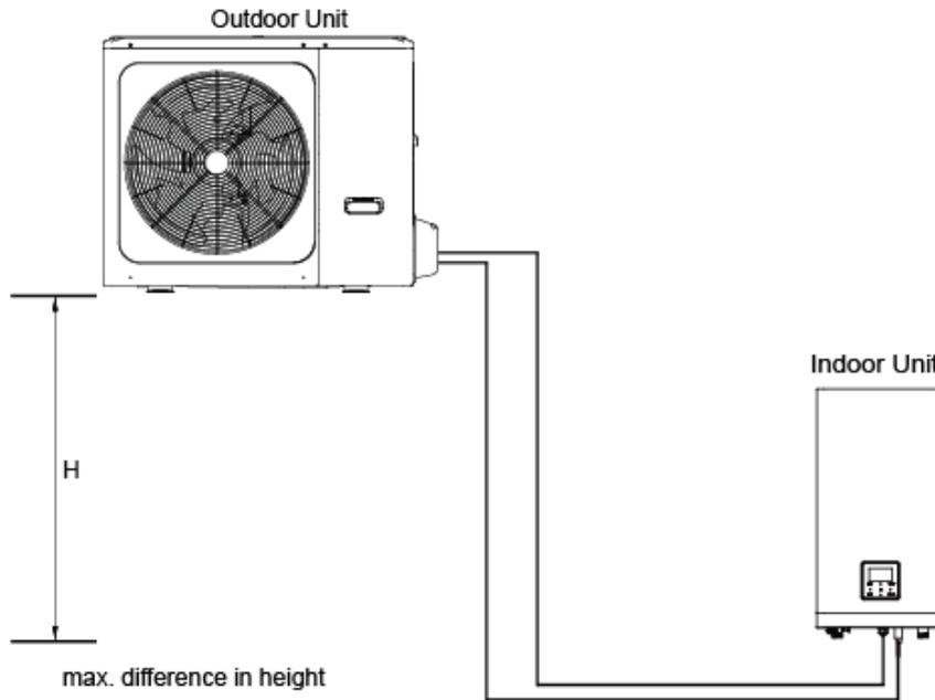
The largest level difference between indoor unit and outdoor unit should not exceed 20m.
