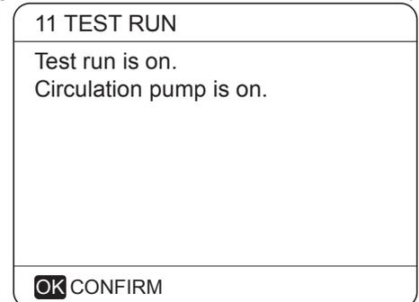
will operate. After a further 2 min the flow switch start to check the water flow. If the water flow rate is sufficient, both PUMPI and PUMPO operate until the next command is received. If the water flow rate is insufficient over any 15-second period, PUMPI and PUMPO stop and error code E8 is displayed. Refer to Part 3, 8.2 "Error Code table".
