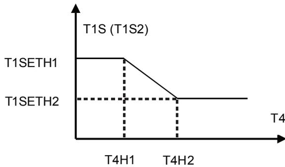
Figure 3-12.7: Automatic setting curve for cooling mode
