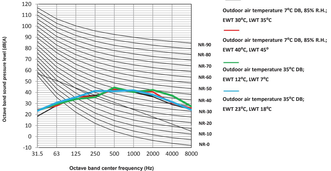
Figure 2-8.4: ATS08S octave band levels
