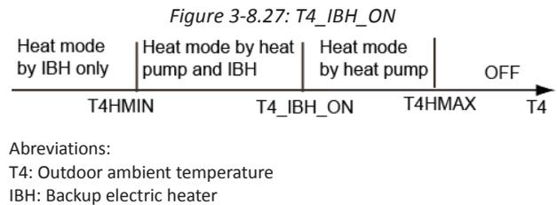
**dT1\_ASH\_ON** sets the temperature difference between the heat pump’s leaving water set temperature (T1S) and the heat pump’s leaving water temperature (T1) above which the additional heating source is on. When  $T1S - T1 \geq dT1\_AHS\_ON$  the additional heating source is on.
