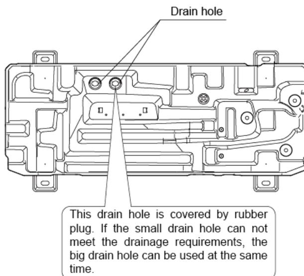
Figure 3-2.5: 8-16kW models drainage hole
