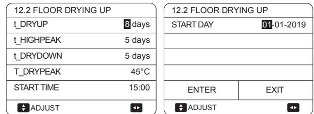
Figure 3-8.45: FLOOR DRYING UP settings
