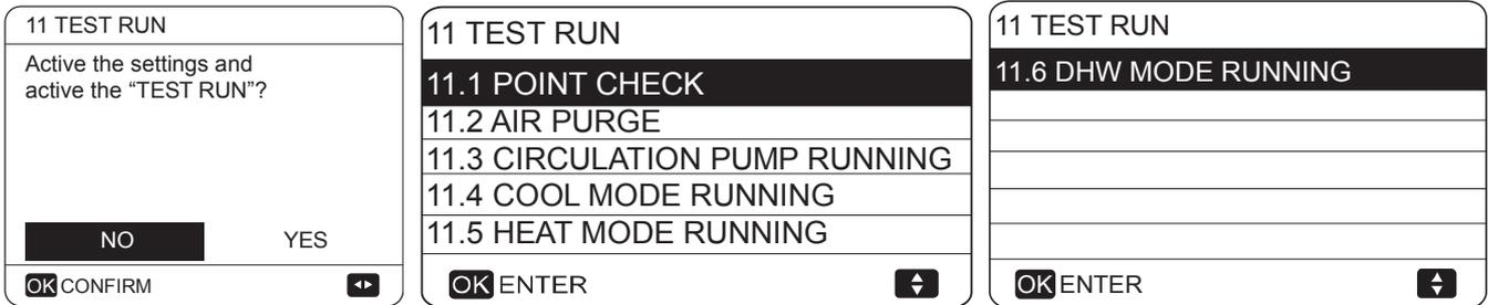
During test run, all buttons except OK are invalid. If you want to turn off the test run, please press OK. For example ,when the unit is in air purge mode, after you press OK, the following page will be displayed:
