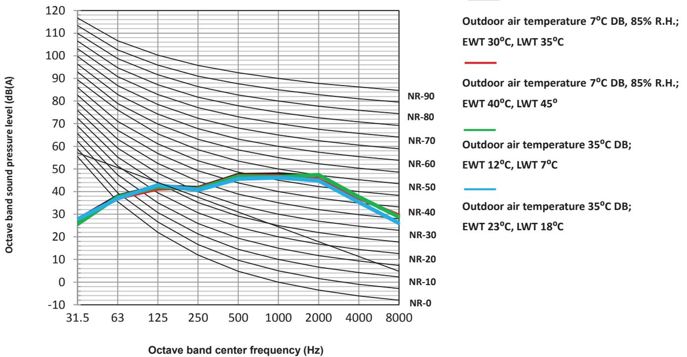
Figure 2-8.5: ATS12T octave band levels
