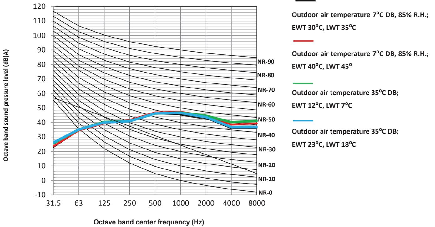
Figure 2-8.5: ATS14T octave band levels
