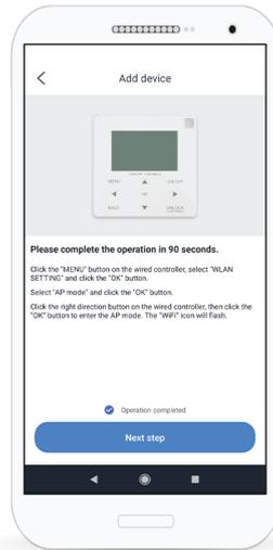
**Step 12.** On the wired controller, select “MENU”, then “WLAN SETTING” and press “OK”. Select “AP mode” and press ok. Click once the right button to selecty the “OK” command, and please “OK” to enter the WiFi mode. The WiFi icon on the wired controller will start flashing. Make sure you complete the operation in 90 seconds after the icon starts flashing. Check the “Operation completed on the bottom part of the screen of the mobile/tablet, and select the “Next step” to continue”.
