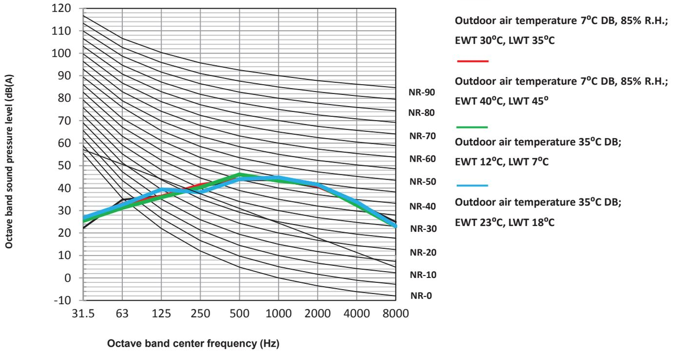
Figure 2-8.5: ATS10S octave band levels
