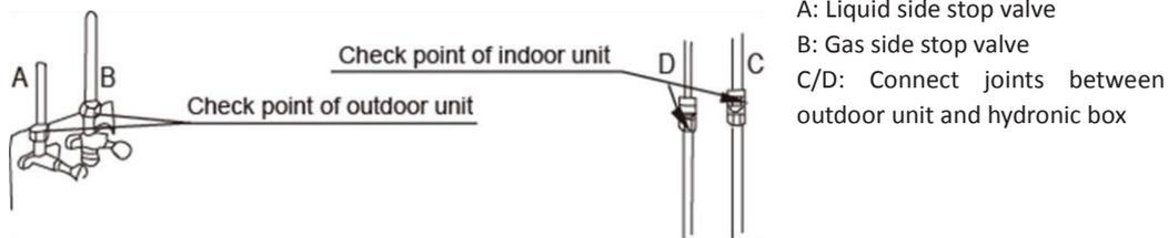
4. Refrigerant leak detection: for leaks that are difficult to detect, refrigerant leak detection may be used as follows:
