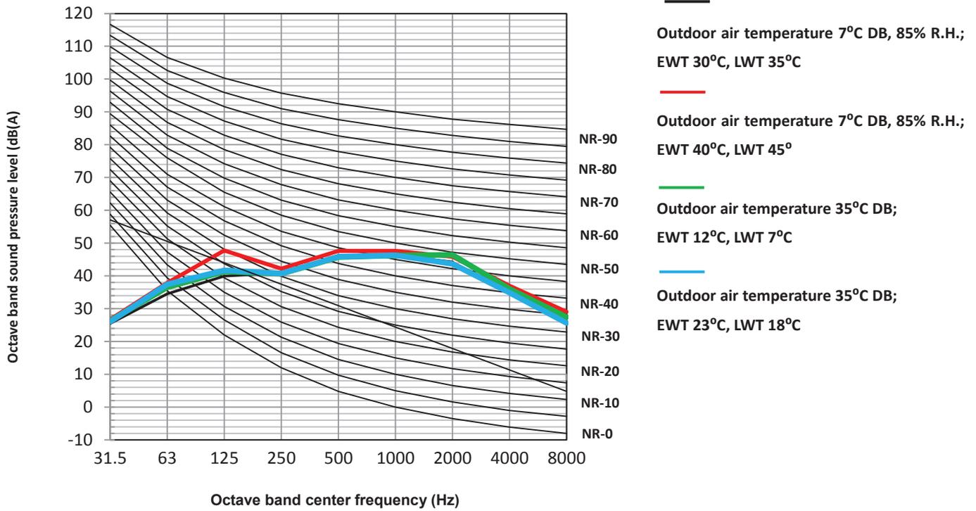
Figure 2-8.5: ATS14S octave band levels
