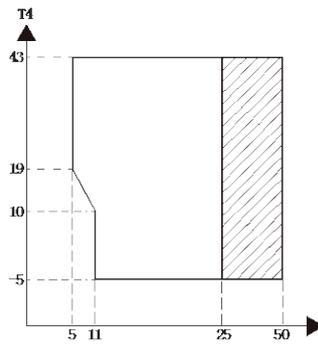
Figure 2-6.3: Domestic hot water operating limits<sup>1</sup>
