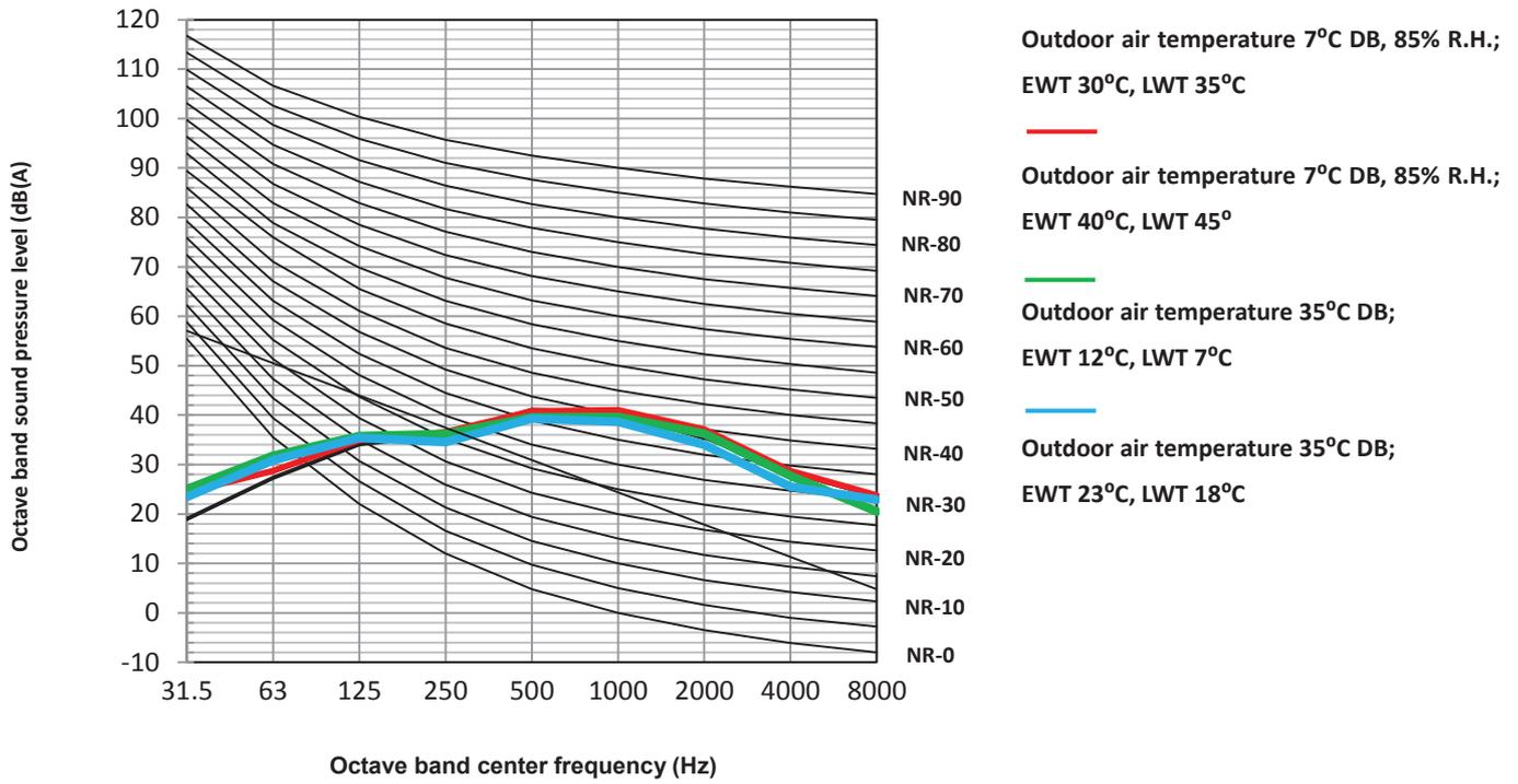
Figure 2-8.3: ATS06S octave band levels
