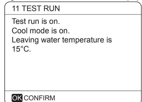
During the **COOL MODE RUNNING** operation, the Matrix Split unit leaving water set temperature is 7°C. The current actual leaving water temperature is displayed on the user interface. The unit operates until the leaving water temperature drops to the set temperature or the next command is received.
