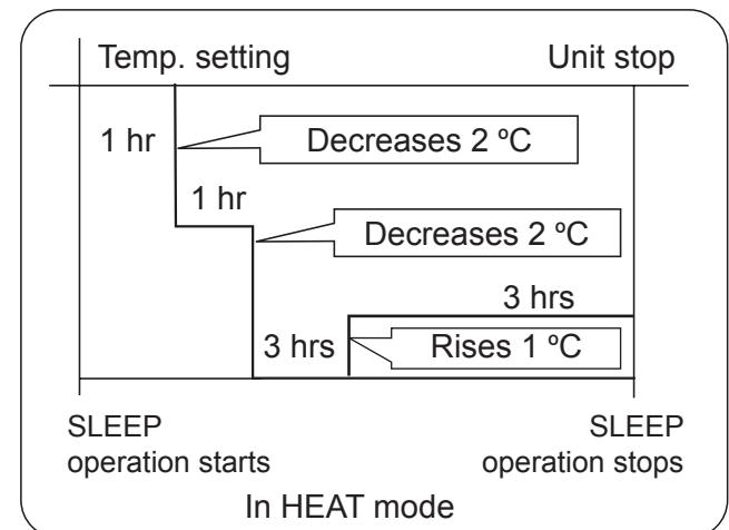
4. When SLEEP mode is set to 8 hours the time can not be adjusted. When TIMER function is set, the SLEEP mode can't be set up. After the SLEEP mode is set up, if user resets TIMER function, the SLEEP mode will be cancelled; the machine will be in the state of timing-on, if the two modes are set up at the same time, either of their operation time is ended first, the unit will stop automatically, and the other mode will be cancelled.
