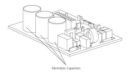
For other models, connect discharge resistance (approx.100 $\Omega$  40W) or a soldering iron plug between the positive and negative terminals of the electrolytic capacitor. The terminals are located on the bottom surface of the outdoor PCB.
