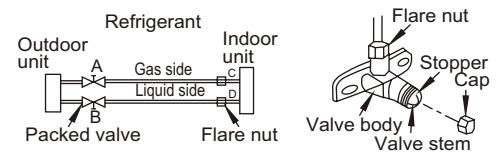
**2. When using the Vacuum Pump**
