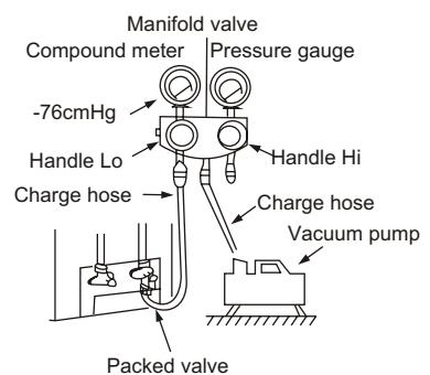
**3. Safety and leakage check**
