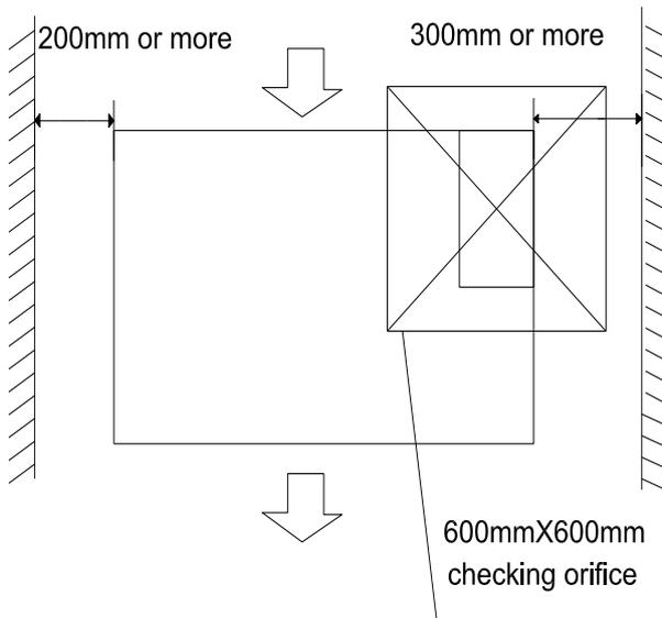
All the indoor units reserve the hole to joint the fresh air pipe. The hole size as following:
