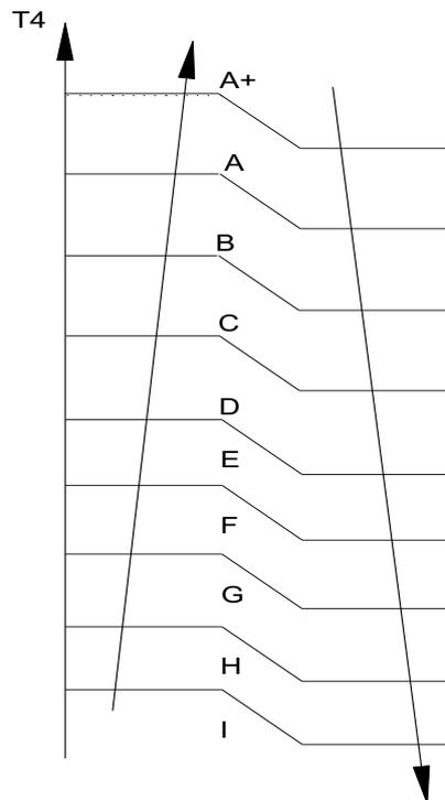
While A,B,C...means different fan speed of outdoor unit.
