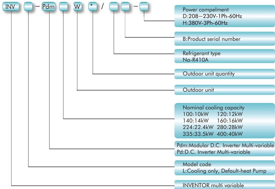
Example: INV-Pdm1700W4/NaB-H:D .C.Inverter Multi-variable outdoor unit of INVENTOR,with 4 outdoor units and the nominal cooling capacity is 170kW. The power supply is 380V-3Ph-60Hz.
