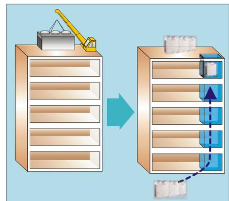
If necessary, installation can be performed by floor. The installers do not have to wait until the entire system is installed in the building to test the system in each section.
