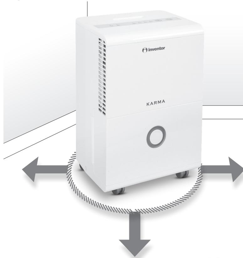
1) Do not block or restrict the airflow around the unit. Make sure the air inlet/exhaust grills are not obstructed. Allow 20cm of clearance around the unit and 40cm above.
