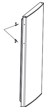
Step 2: Install the door handle to the door and fasten it with screws
