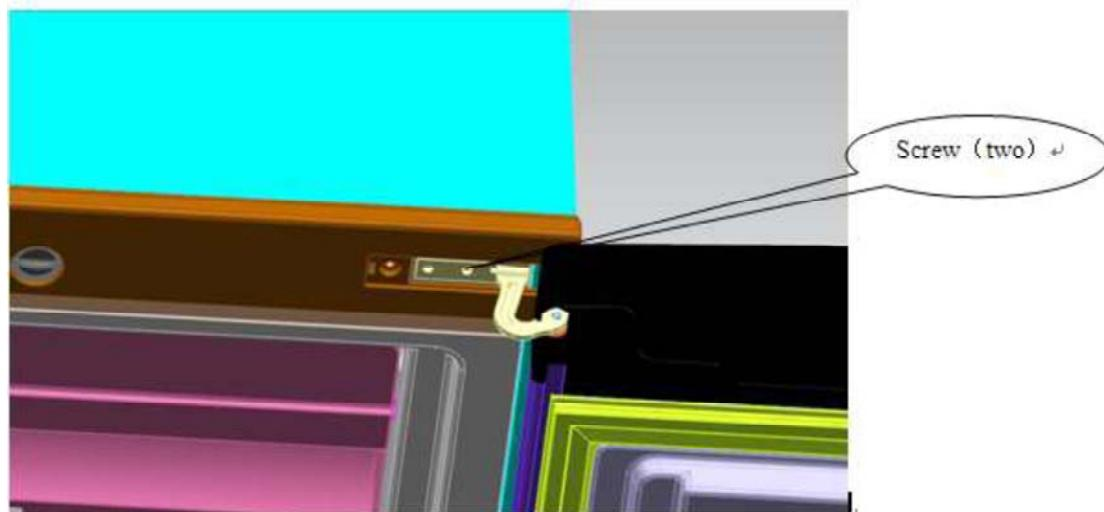
3) Replace the top-hinge and the top-door limit block and the door bearing bush to the other side.
