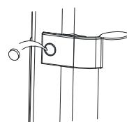
Step 3: Cover screw caps of the handle into screw holes
