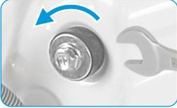
Loosen the 4 transport bolts with a spanner.
